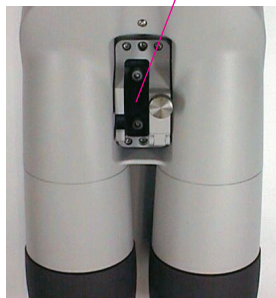
1-2. Installation of the Mount Block
