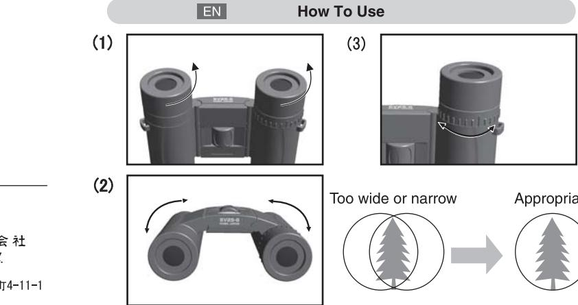
To ensure the maximum performance of the binoculars, you must first adjust them to your own visual acuity. This is achieved by adjusting the eyecups and interpupillary distance, setting the diopter, and adjusting the focus. Image visibility differs according to your physical condition, surrounding environment, and weather conditions.
